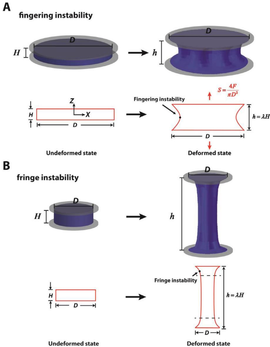
**Fig. 1.** (a) Schematic of the formation of fingering instabilities in elastic layers with diameter of  $D$  and thickness of  $H$ . Fingering instability initiates at the middle-plane of the elastic layer. (b) Schematic of the formation of fringe instabilities in elastic layers with diameter of  $D$  and thickness of  $H$ . Fringe instability initiates at the plane close to the fringe portion of the elastic layer. The aspect ratio of the layer is defined as  $\alpha = D/H$ .
