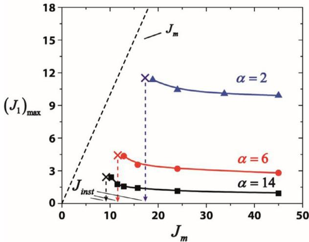
Fig. 6. The maximum strain invariant  $(J_1)_{\max}$  at the plane where instability initiates with various limit of first strain invariant  $J_m$  and aspect ratio of  $\alpha=2$ ,  $\alpha=6$  and  $\alpha=14$  at the onset of instabilities.
