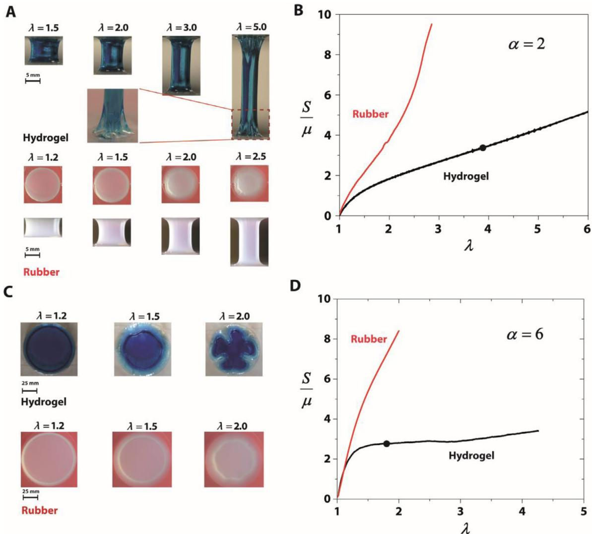
**Fig. 9.** Experimental validation of the suppression of fingering and fringe instability in a stiffening layer. (a) The evolution of the deformation in a hydrogel layer and rubber layer with aspect ratio of  $\alpha = 2$  and (b) corresponding applied stress-stretch curves. (c) The evolution of the deformation in hydrogel layer and rubber layer with aspect ratio of  $\alpha = 6$  and (d) corresponding applied stress-stretch curves. Dots represent the onset of the instabilities.
