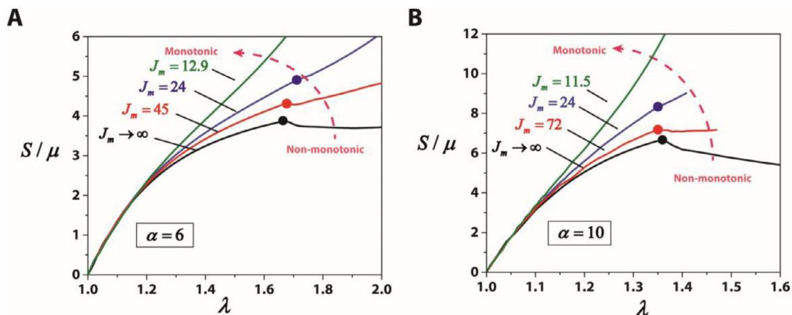
Fig. 7. The stress-stretch curves for the sample with (a) aspect ratio of  $\alpha = 6$  and (b)  $\alpha = 10$ . Dots represent the onset of fingering instabilities.
