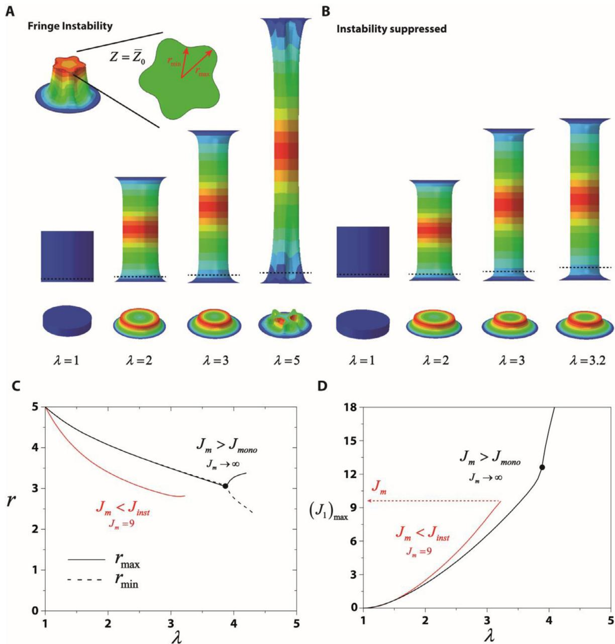
**Fig. 5.** Suppression of fringe instability in the sample with aspect ratio of  $\alpha = 1$ . (a) Fringe instability emerges in a neo-Hookean layer. (b) Fringe instability suppressed in a Gent solid with the limit of the strain invariant  $J_m = 9$ . (c) The radius of the outer surface at the plane  $\bar{Z}_0 = 0.9$  where undulations initiate and (d) the maximum first strain invariant  $(J_1)_{\max}$ . Dots represent the onset of fringe instabilities.
