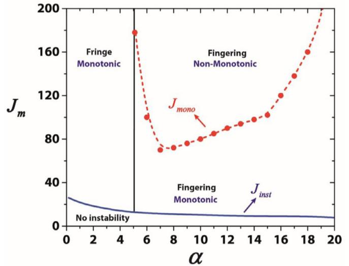
Fig. 8. A phase diagram elucidating the suppression of fringe or fingering instabilities and the stress vs. stretch relation in confined elastic layers with respect to layer's aspect ratio  $\alpha$  and limit of the strain invariant  $J_m$ .
